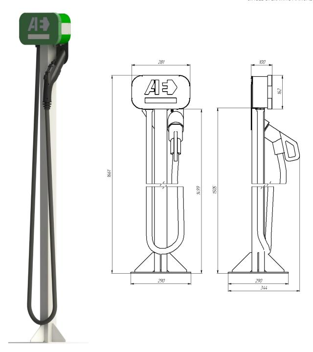
Figure 1b - Appearance and dimensions of the Station for floor mounting
