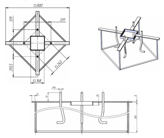
Figure 3 – Appearance and dimensions of the insert
