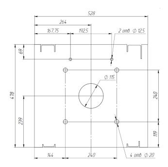
Figure 4 – The pedestal foundation (bottom view)
