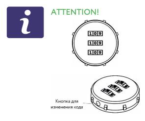
A digital security lock is used. The default lock code is "000".
