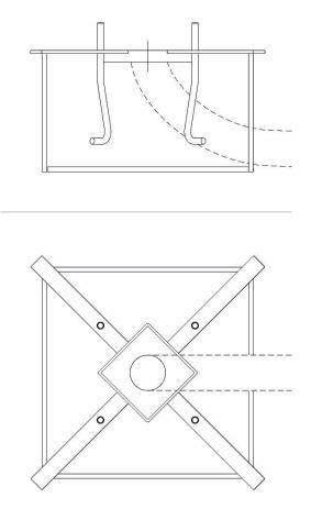
Figure 5 – The Station foundation
